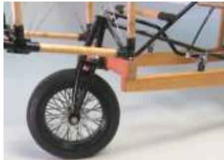
Photoetched front wheel and mounting details
