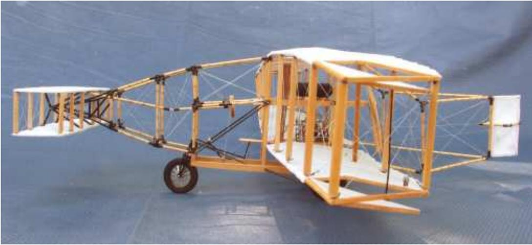
attached to a U shaped yoke that passed around the pilot, just under his arms. To bank the plane, he just leaned slightly in the direction he wanted to go, much like a motorcycle or skiing.
