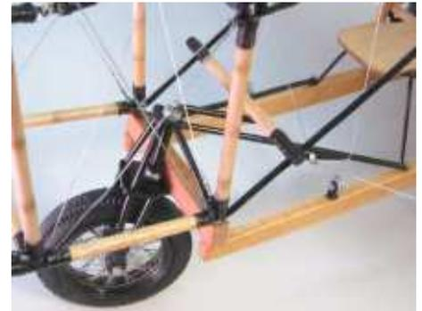
Front wheel steering mechanism and pilot's "footrest"
