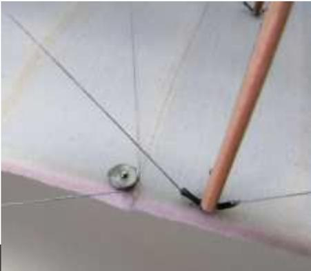
Details of a lathe turned pulley for the rudder cable, some of the more than 140 scratchbuilt brackets
