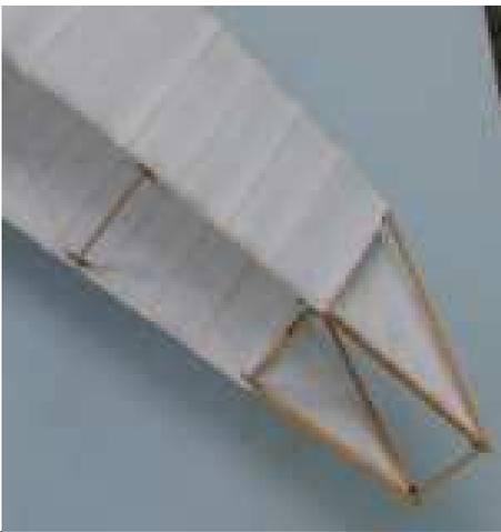
The pair of outboard mounted triangular ailerons
