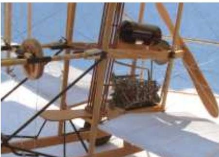
Combined gas and oil tank mounted above engine
