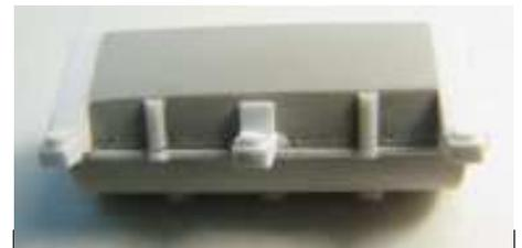
(Above and below) The engine block built up from styrene
