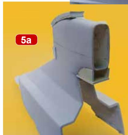
between. **Photos 5 and 6** show some of the intermediate progress steps. During final dry assembly, it became apparent that the roll bar would interfere with the lowered front of the scoop. Luckily this was caught in time and was easy to
