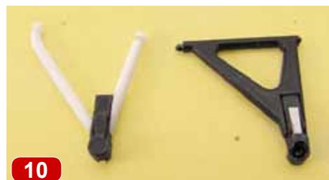
allowed the suspension to work. The moulding seams on all the linkages and the joint on the rear uprights were all cleaned up and prepped for the same paint as the front suspension.
