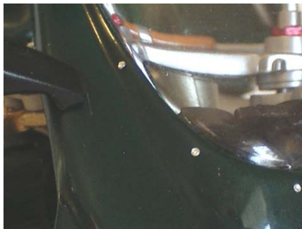
Figure 8 - Rivets around windscreen
